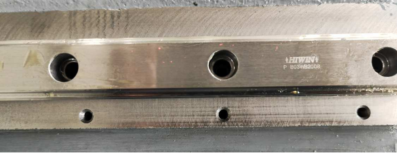
HIWIN “P” grade linear guideway for guide for X,Y,U,V and “H” grade for Z axis
