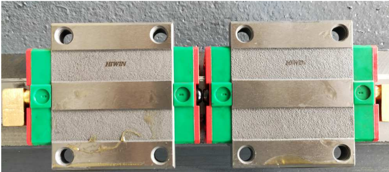
HIWIN “P” grade linear guideway for guide for X,Y,U,V and “H” grade for Z axis
